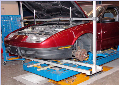
One of four recessed Car-O-Liners with mechanical measuring systems
